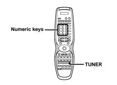
**1** Press the TUNER key to select tuner as the source.
