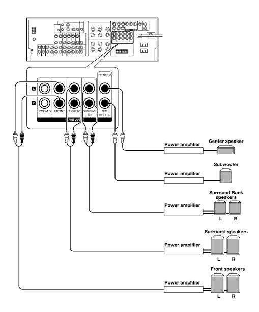
• Connecting a speaker cord directly to a **PRE OUT** jack will not produce any sound from the speaker.
