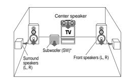
\* LFE = Low Frequency Effects. This channel delivers separate nondirectional bass singnals to the subwoofer for more dynamic deep bass sound effects.
