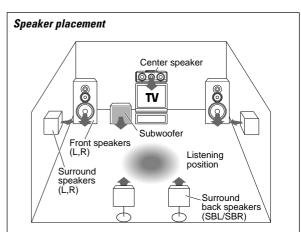
Front speakers : Place at the front left and right of the listening position. Front speakers are required for all surround modes. Center speaker : Place front and center. This speaker stabilizes the
