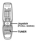
**1** Press the TUNER key to select the tuner as the source.
